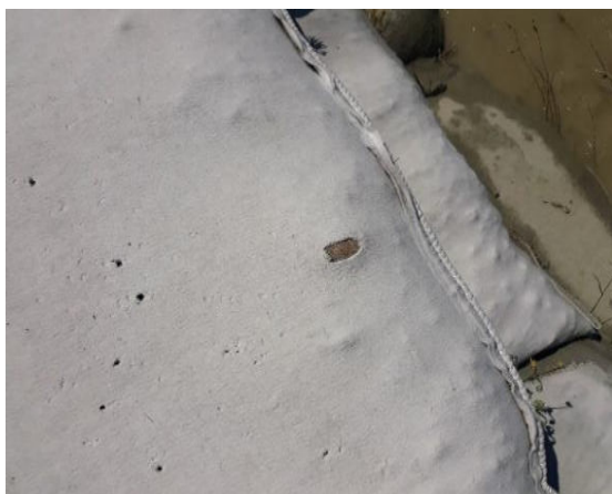
Figure 46. Degradation caused by sharp or angular objects (author's photo)
