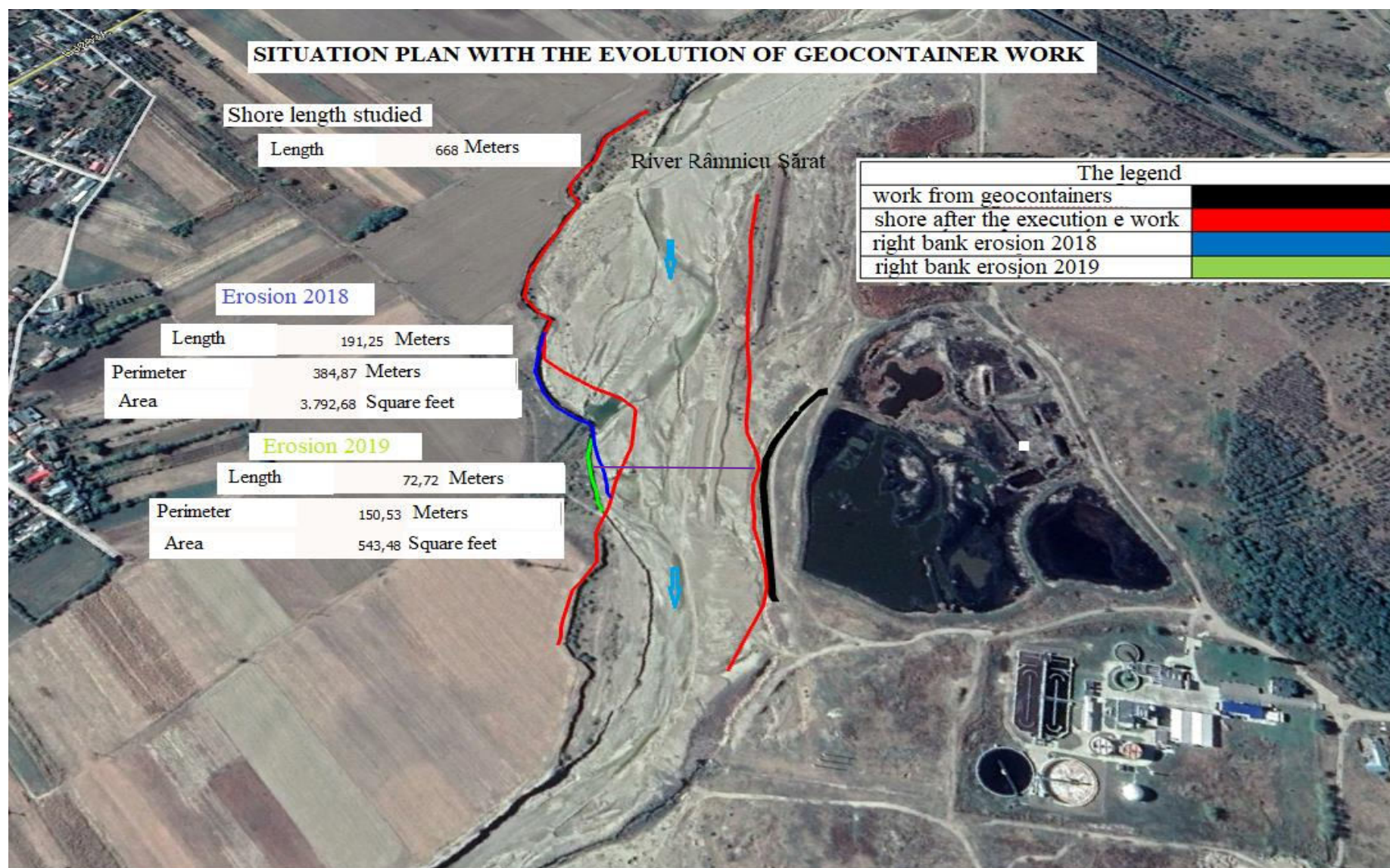
Figure 48. The evolution of the work in geocontainers in the period 2018-2019
