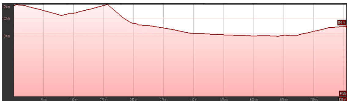
Figure 74. Transversal profile through the Milcov riverbed in 2019 after the execution of the work
